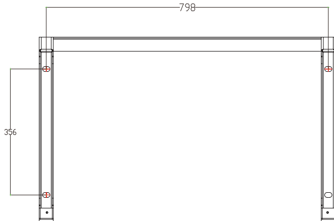
Pic 4.4 Mounting bracket dimensions
